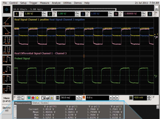
Figure 14. Scenario 9, Function generator is set to slow square wave, 3.3 Vp-p, 0-V offset.
