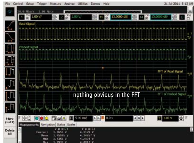
Figure 21. Examining the spectra of a square wave to determine if a probe amplifier is in compression.
