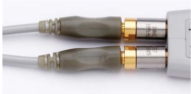
Figure 17. Inline attenuators used with an InfiniiMax I or II probe head.
