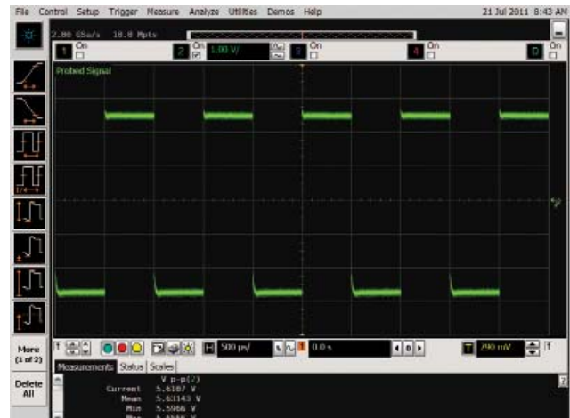
Figure 22. Comparison of a probed square wave. The one on the left is in compression. The rounded corner is the only telltale sign.
